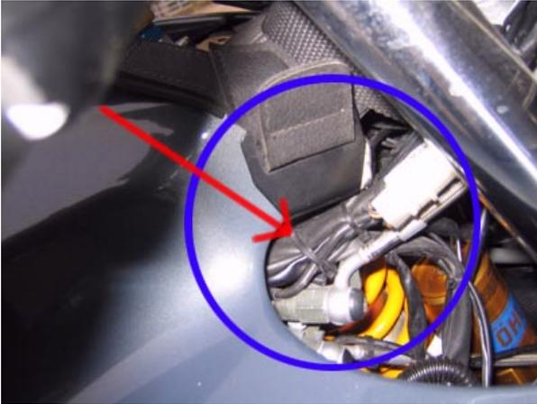
**1.** If necessary cut the cable ties that fasten the handlebar control wiring harnesses near the stock bars and at the steering head.
