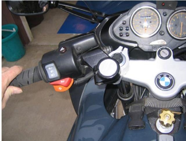
**7. Alignment:** Most people like to align the bar backs parallel and symmetrical, tighten, and then adjust the comfort bars to suit. However, the barbacks have some concentric adjustment on the fork tube. Use your own discretion and adjust the set-up to fit your ergos best. Adjust the barbacks and comfort bars to clear the fuel tank at full steering lock in both directions.
