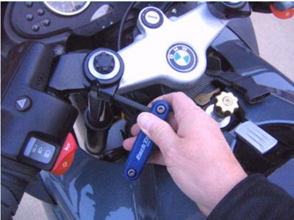
**3.** Loosen the socket head cap screws completely and remove the comfort bars from the fork tubes on one side. Place it on some padding like a towel, on top of the fuel tank to avoid scratches. Clean the surfaces of the fork tubes to remove any dirt, grease and oil.
