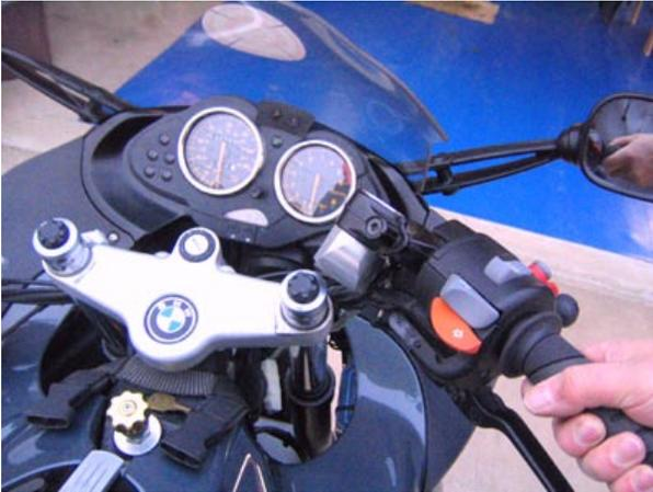
5. **\*Second!** Mount the entire handlebar and barback assembly onto the fork tube. You'll find this is much easier than trying to mount the barbacks first and *then* stretching your wires and cables to get the comfort bars onto the barback's post. Repeat steps 1-5 on the other side.
