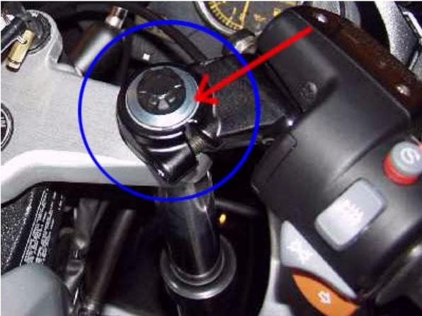
**2.** If you haven't already raised your bars on the fork tubes like I did, remove the wire circlip that holds the bars on. Put the circlip in your parts drawer. You won't be needing this.
